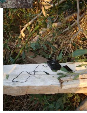
Mini tape lure equipment with device of tape and loudspeaker and a battery for a few hours
